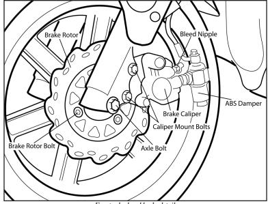
Front wheel and brake detail.
