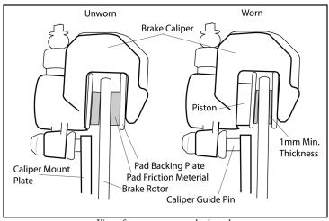
View of worn vs un-worn brake pads.
