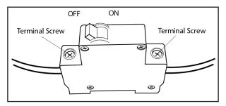
The main breaker has two functions – to protect your MOTORINO™ from excessive damage due to an electrical fault, and to act as a complete disconnect from the battery pack. The breaker is located under the seat on models with an enclosed storage compartment, and under a locking panel in the floor of the XPd.
